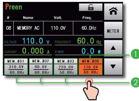
To create a complex sequence on the HMI is no longer a difficult task for AFV-P series. The 5 inches touch screen provides users a clear display and an easy set up. AFV-P series can display 4 shortcuts of Memory Sets, and the voltage and frequency setting of each Memory Sets can be clearly read. The user can quickly switch the output by selecting the shortcuts.
