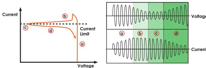
When it comes to over current, AFV-P series offers more than just shutdown protection. Over current foldback enables AFV-P series to maintain the output current at the rated current and correspondingly decrease the output voltage as the load impedance increases. It is an extended protection or an alternative to provide constant current for EUT.
