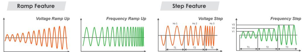
Ramp and Step feature allows users to define slew rate of voltage and frequency at each Step. Users can set the rise/fall time, time unit and voltage/frequency change between Steps to create a wide range of waveform. Additionally, Ramp feature can effectively reduce the inrush current by simulating soft start for motor or compressor startup.
