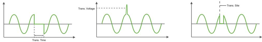
Through the Transient feature, user can have more control over the waveform by inserting disturbance at user-defined locations with user-defined drop/rise range. This is a useful feature to simulate different pre-compliance tests and various types of power line disturbance, such as surge, sag, spike and dropout, for immunity tests.
