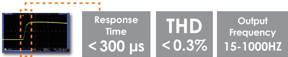
AFV-P series is a high performance AC power source with fast response time, low total harmonic distortion and tight voltage regulation. With its technically advanced features, users can easily simulate power line disturbance, such as sags, surges, dropouts and spikes.
