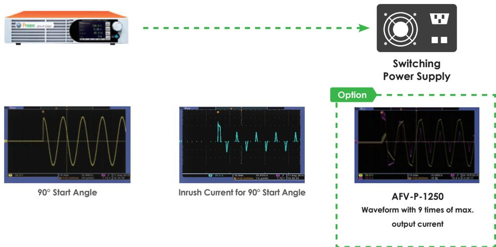
For switching supply (rectified load), AFV-P series provides standard inrush current as 4.5 times of max. output current and the AFV-P-600 and AFV-P-1250 have optional 9 times of max. output current, which makes AFV-P series the lowest capacity in the market that can achieve the highest inrush current. Moreover, the AFV-P series allows users to set the start angle/end angle for the product output, which is suitable for testing switching power supplies.
